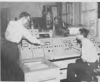
IMPROVED INSTRUMENTATION such as the mass spectrometer, above, is a constant tool of research men. The apparatus at right is used to conduct new tests on catalysts. Basic purpose of the device is to study the distribution of active sites on catalysts so that high octane gasoline can be refined as effectively as possible.
